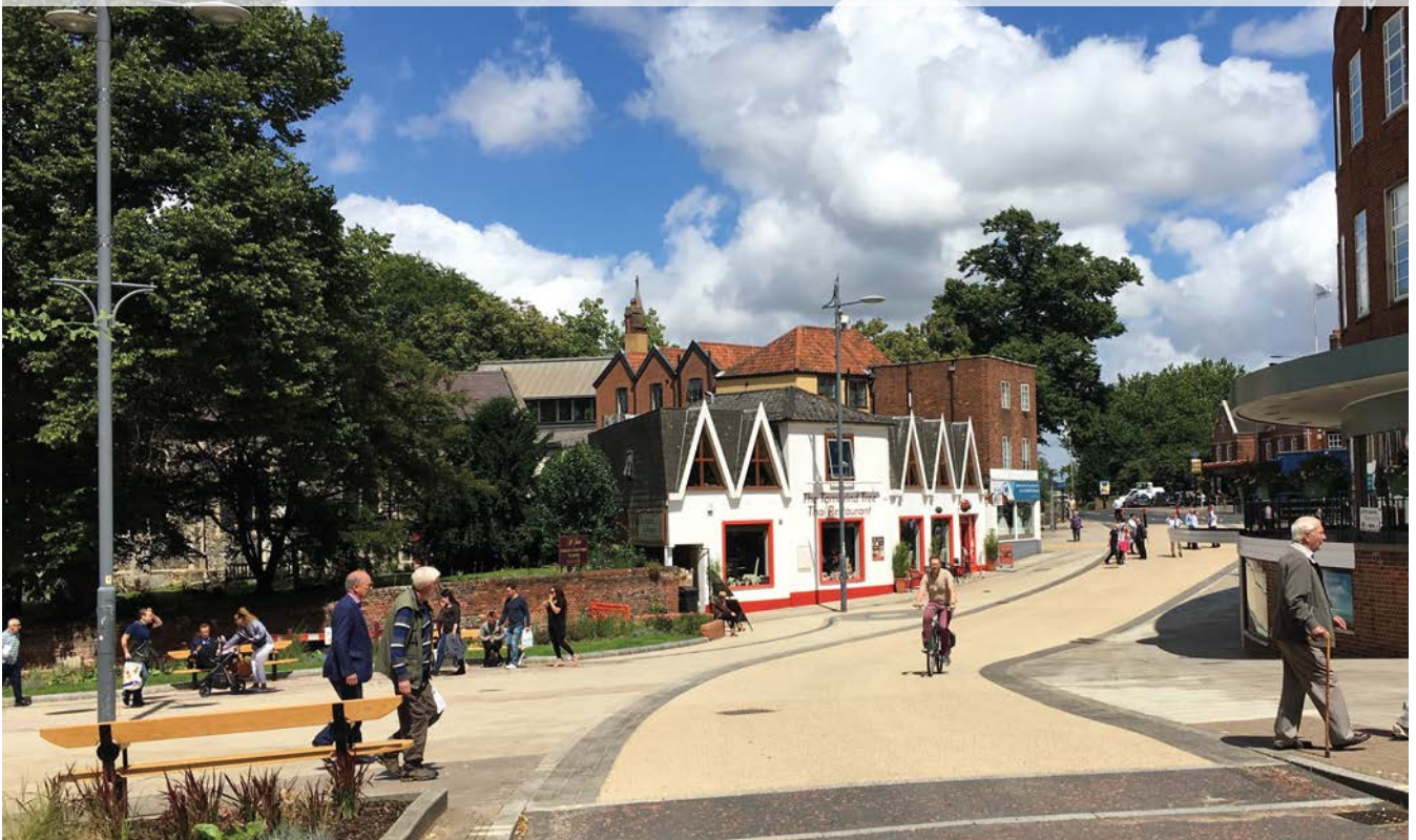
Figure 4.4: City centre access road, Norwich, uses a mode filter and vehicle restricted area to provide separation from motor traffic
