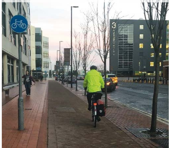
Figure 6.14: Cycle track with sign to TSRGD diagram 955
