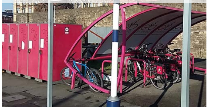
Figure 11.7: Multi-purpose cycle hub within a railway platform: secure lockers for regular users, plus covered stands to accommodate ad hoc users and Northern Rail’s “Bike-n-Go” cycle hire vehicles
