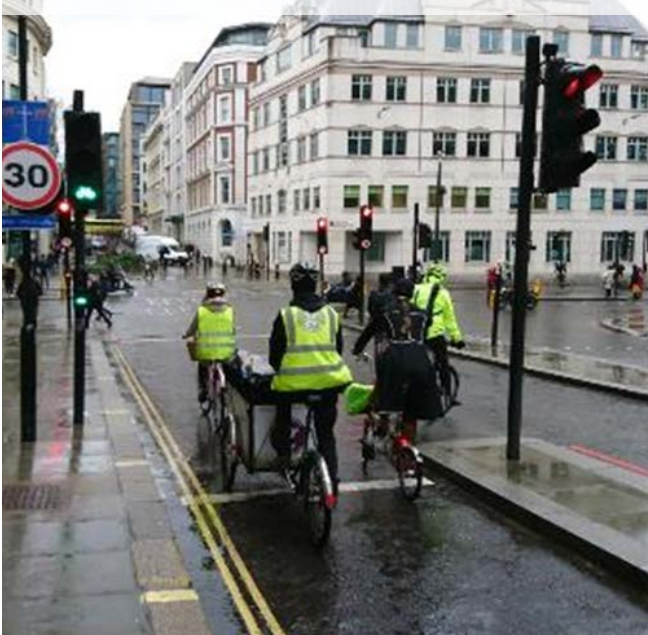
Figure 10.32: Cycle gate, Southwark Bridge, London
